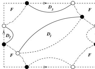
Figure 3.4: Three dipoles incident with the same face
